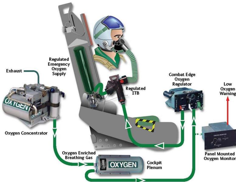
OBOGS eliminates the need for LOX by utilizing bleed air from the engine and separating its components through a two-bed molecular sieve pressure swing adsorption (PSA) technology.
