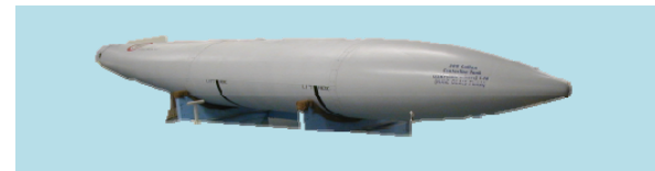
300gal Centerline Tank PN: 2-300-48302-SERIES
