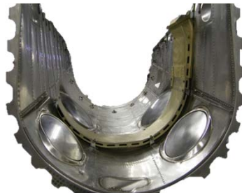
Inboard Nacelle Completed Assembly
