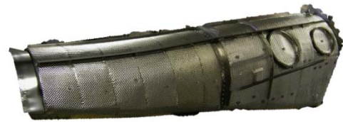
Inboard Nacelle Forward & Mid Sections
