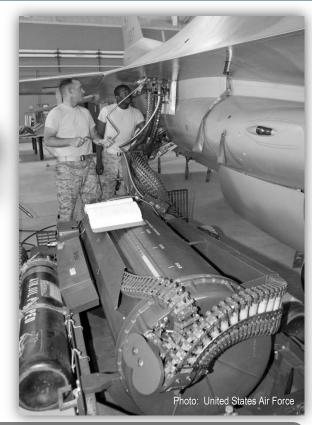
The UALS's 2100 round capacity loads either four F-16, two F-15, or three F/A-18 aircraft before it must be replenished.
