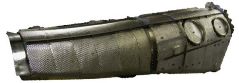
Inboard Nacelle Forward & Mid Sections
