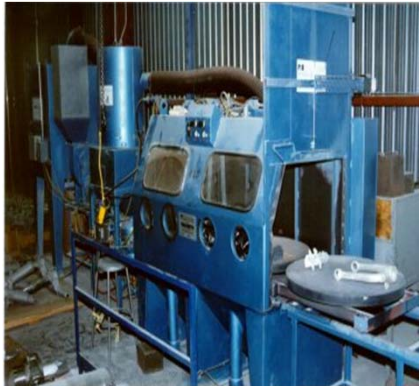
PLASTIC MEDIA BLASTING
