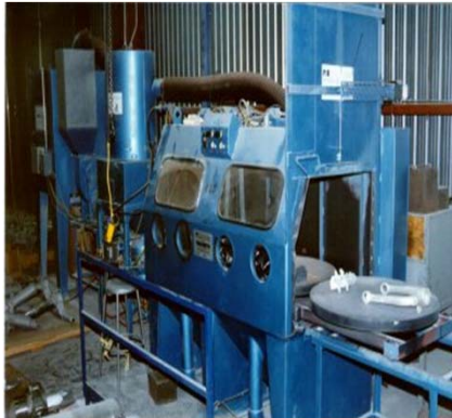
PLASTIC MEDIA BLASTING
