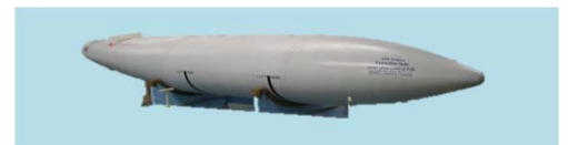
300gal Centerline Tank PN: 2-300-48302-6 / NSN: 1560-01-287-4583
